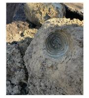
New Rockford got its name for a reason! Just as the sandy and rocky soil underneath us creates issues for farmers and builders, the directional drilling machine can also become a victim to it. The photo above shows what happens when the metal rod hits a rock! Spoiler alert: the rock wins!
